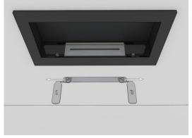
Then, by continuously sliding the two handles outwards, move the cover over the burner and cover the opening from which the flame is coming. This should be done evenly and simultaneously for the entire width.
